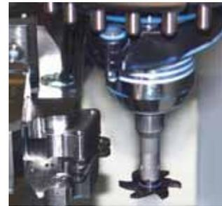
Picture, top: The slots are milled in the two jaw sections with the slot miller 636.
